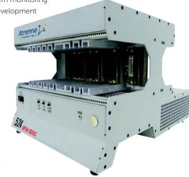
The 524 Open Series development system can be configured with a power control module (PCM). The PCM provides system fan speeds, DC voltage outputs, and monitoring for temperature sensors. External access to the PCM is available through a rear-mounted Ethernet connector or RS-232 port.
