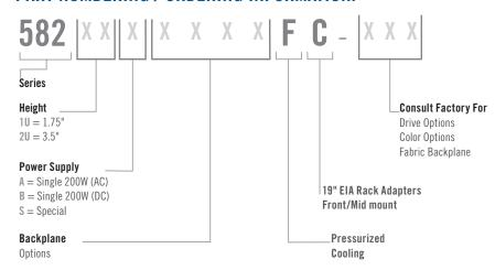
**Example:** 5821SSPBPFC-100 is a 582 Series, 1U high with one 200W DC input power supplies, 4-Slot hot swap, right justified backplane with H.110 bussing and 5V keys installed. One Intel ZT 7102 alarm card.
