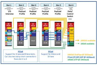
The four Module Profiles ending in "-n" in the table above indicate that VITA 65.1 currently does not have any profiles supporting 16 Gbaud PCIe Gen4 nor 25.78125 Gbaud 100GBASE-KR4
