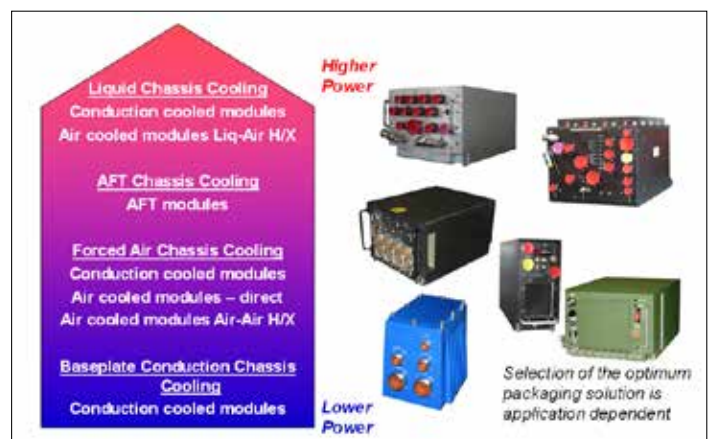
Figure 4: Chassis Mechanical and Cooling Options
