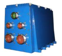
The Small Form Factor-6 (SFF) utilizes an ATR-style design for maximum baseplace conduction cooling. Engineered for strength, lightweight, and maximum cooling in a conduction-cooled environment, the SFF-6 enclosure incorporates a specially designed frame and configurable conducting walls for extended temperature, shock and vibration protection.
