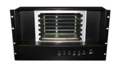
The DT-CC is a horizontally-oriented, rackmount/desktop chassis for high-powered, 6U, conduction-cooled VPX modules. Horizontal air-flow cools over 150W per slot to support state-of-the-art processor boards.
