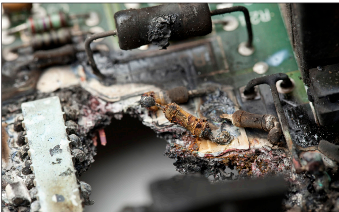
Results of inadequate cooling
